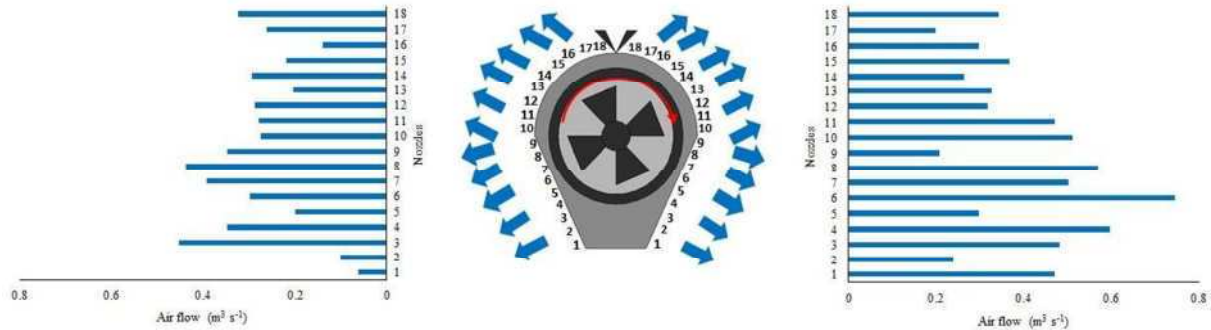
4 5 Figure 1. Distribution profile of airflow from the hydraulic nozzles of both sides of the axial 6 fan sprayer.
