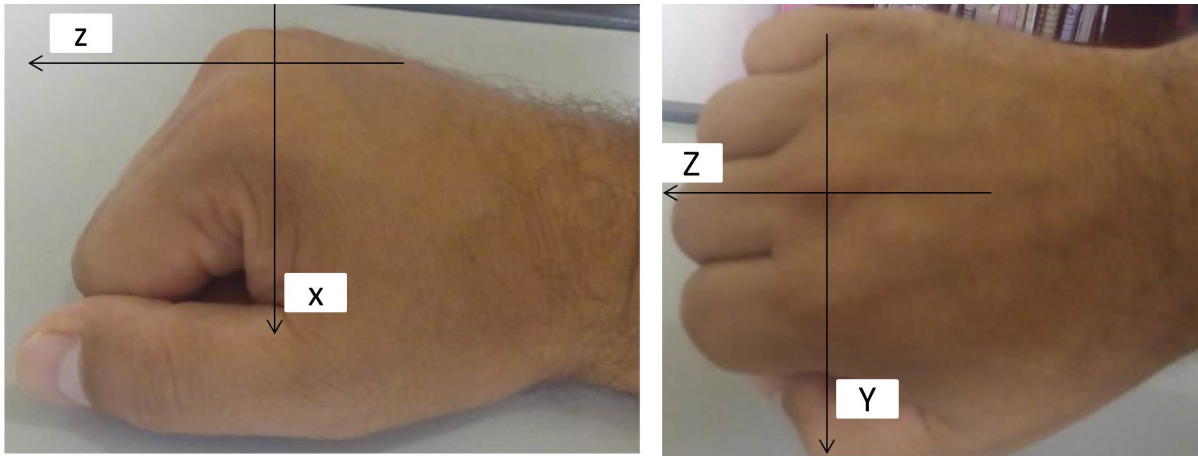
FIGURE 5 - Direction of the Orthogonal Axes “x”, “y” and “z” according to NHO 10.
